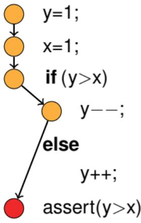
The graph shows the control flow of the main function. It starts at a yellow initial node. The first statement is y=1;, followed by x=1;. Then it reaches an if (y>x) node. If y > x, it goes to a yellow node with y--;. If y <= x, it goes to a yellow node with y++;. Both paths eventually converge to a red final node with the assertion assert(y>x);. Finally, the loop concludes with a closing brace }.
